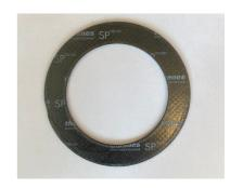
SP <sup>TRD 401</sup> is a gasket material based on graphite with tanged stainless steel sheet insert. The tanged stainless steel sheet insert achieves a higher surface load and protection against blowing out. The material has excellent chemical, thermal and mechanical resistance. Due to its excellent properties, it is used in many industrial sectors, in gas and steam supply as well as in the chemical and petrochemical industry.
